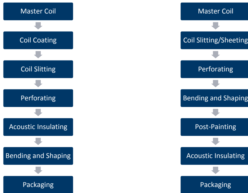
Figure 3-1: Metal specialty product manufacturing process, coil-coating (left) & post-paint (right)
